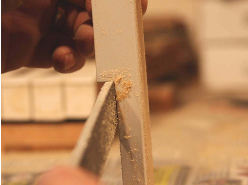
Photo 61: With the keys on the keyframe, a straight edge is clamped down over the keys, using the traditional “dimes-thickness” between the front of the sharps and the back of the notch. An awl is used to mark the cut line, and the excess material is filed out in a two-step process – first with the edge of the file as shown.
