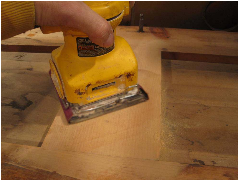
Photo 68: A little time with a hand sander, using 100 grit followed by 150, does wonders.
