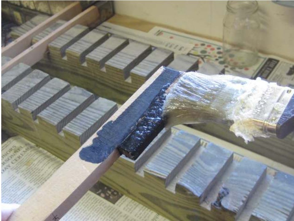
Photo 65: The old lacquer on the sharps is stripped of with commercial stripper. The sharps are hung upside-down in the racks to avoid having the stripper find its way into the bushings on the bottom of the keys.
