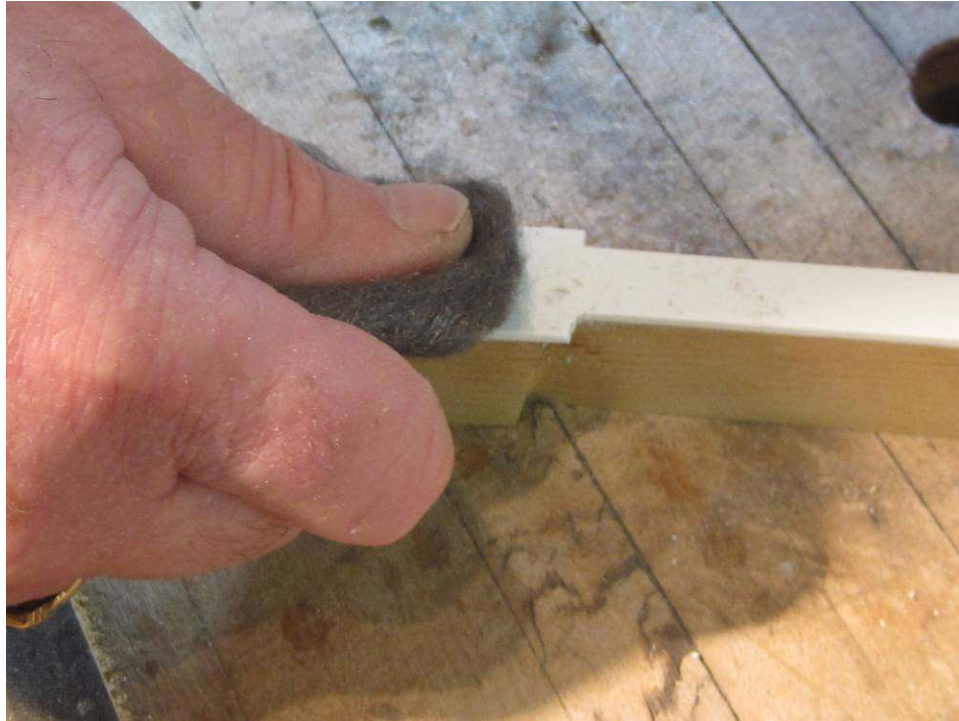
Photo 63: Each key is buffed with 0000 steel wool for a satin finish.
