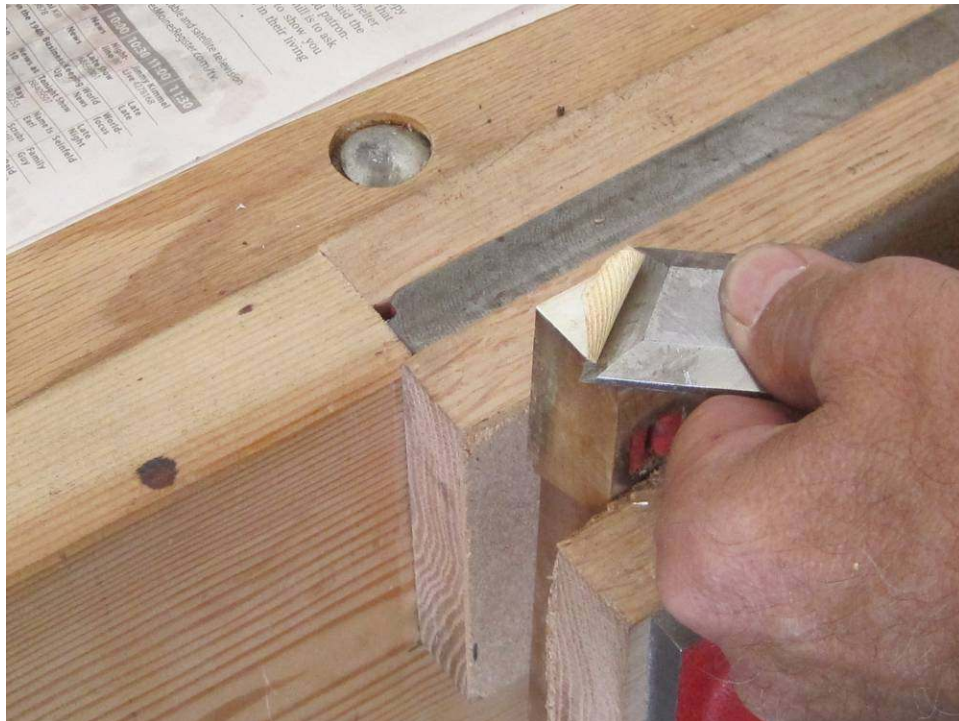
Photo 54: Each key is put in the vise so that the front may be chiseled off.
