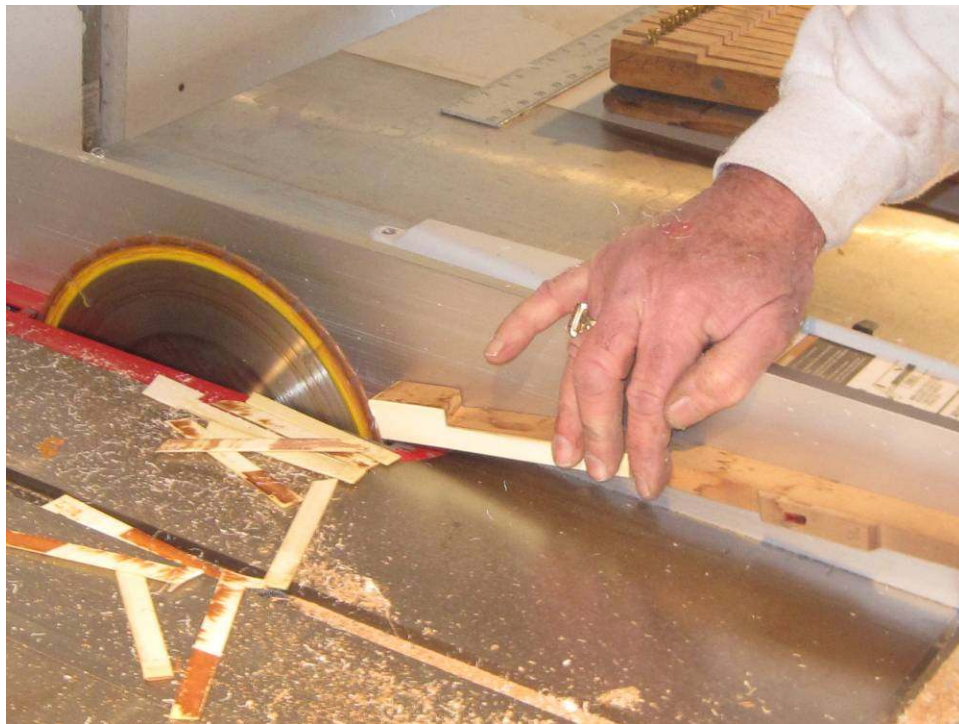
Photo 52: Since there is no ivory to salvage, Dave wastes no time removing the old tops by cutting them off on the table saw. The blade depth is set to remove a fraction of an inch of the wooden keystick to compensate for the thicker German-made keytop material to be installed.
