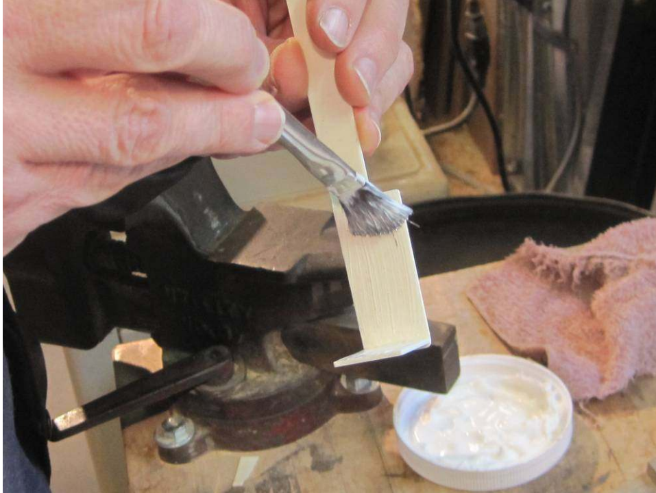
Photo 55: New keytops are coated with PVC-E glue. This glue forms a solid joint without having to be clamped – amazing stuff.
