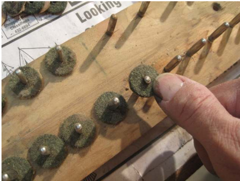
Photo 71: The front rail felts are removed first, using a small flat-bladed screwdriver to lever them off.
