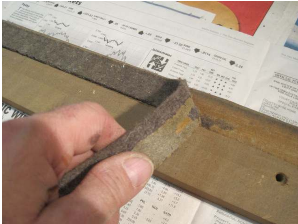
Photo 73: The original back rail felt is first peeled off.
