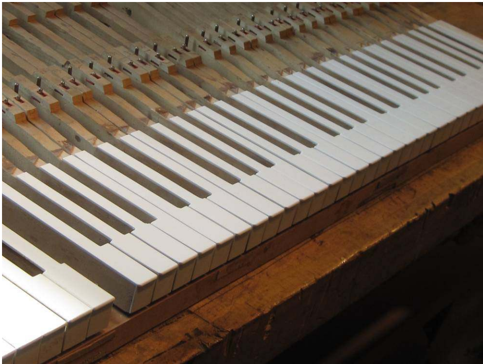
Photo 60: Again, Dave works from one end of the keyboard to the other as he files the sides of each of the keys, this time going from right to left. A close look at the photo reveals uneven notching around the sharps. That will be the next step.
