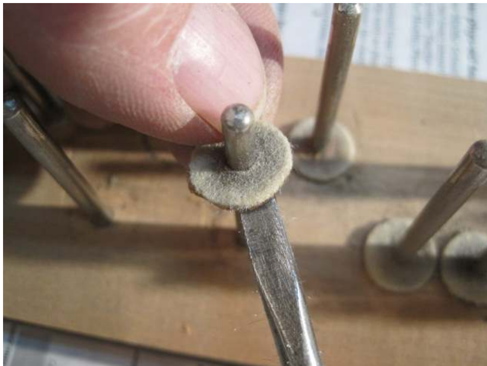
Photo 72: Next come the center rail felts, along with the original leveling papers. By going down to the bare wood, and starting from scratch, a more reliable result will be obtained when the keys are leveled.
