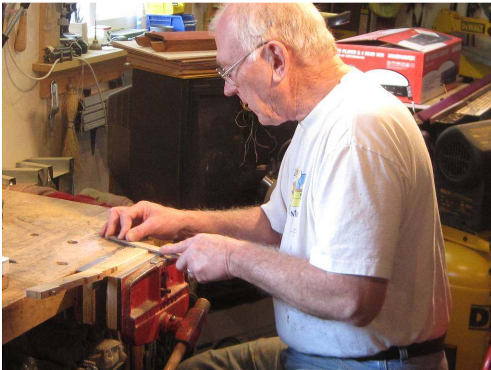
Photo 58: Dave takes advantage of the early morning light the next day to begin filing keytops. Some shops do this with machines. In our shop, we prefer using hand files for a more precise finish.
