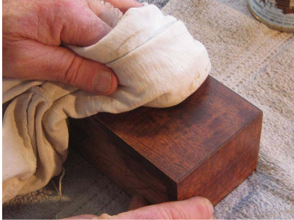
Photo 33: The compound is allowed to dry for a few minutes, then buffed out with a soft rag. All trace of the steel wooling disappears with this final step.
