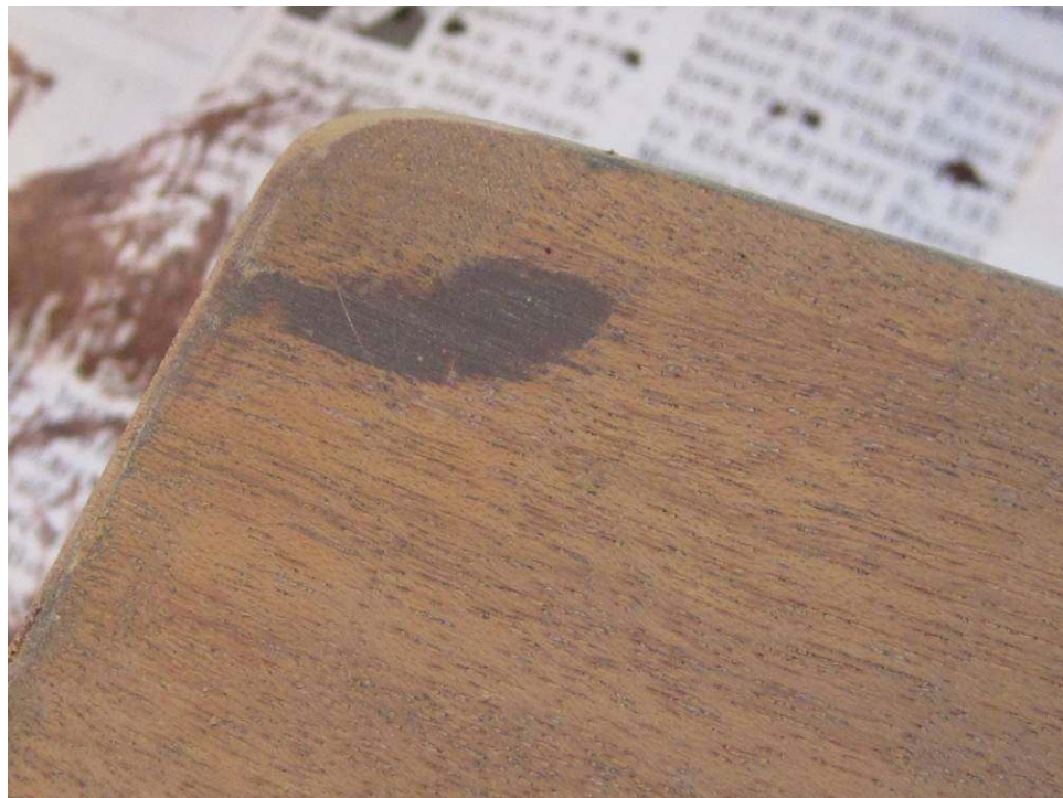
Photo 27: The trick with lacquer stick work is careful slow hand sanding with a fine grit (150 followed by 220). Sanding that is too aggressive will heat the heat and begin to melt the lacquer stick material. Again, this repair will be nearly invisible once the stain is applied.
