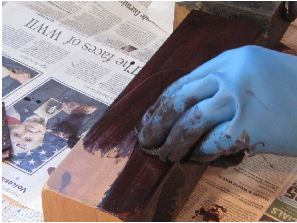
Photo 28: Oil base Minwax mahogany stain is applied to the case and all the parts. This is Dave's favorite step – seeing the transformation as the wood takes the color.
