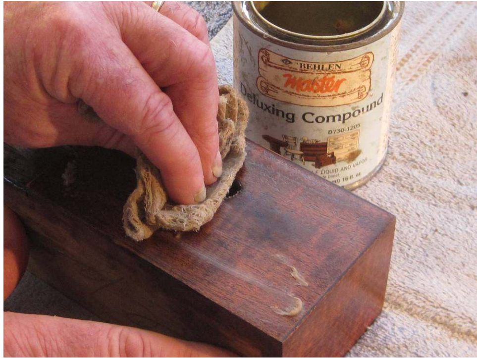
Photo 32: The final step in finishing is an application of deluxing compound. This is somewhat like a paste wax, but is a harder finish, less prone to smearing than paste wax is.
