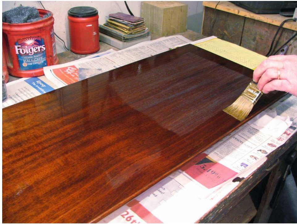
Photo 30: Minwax satin polyurethane is now brushed on to each individual case part. Three coats are applied, with the first and second coat scuff sanded with 600 grit sandpaper to improve adhesion. The final coat is lightly sanded with successively finer grits, finishing up with 1200 grit paper.
