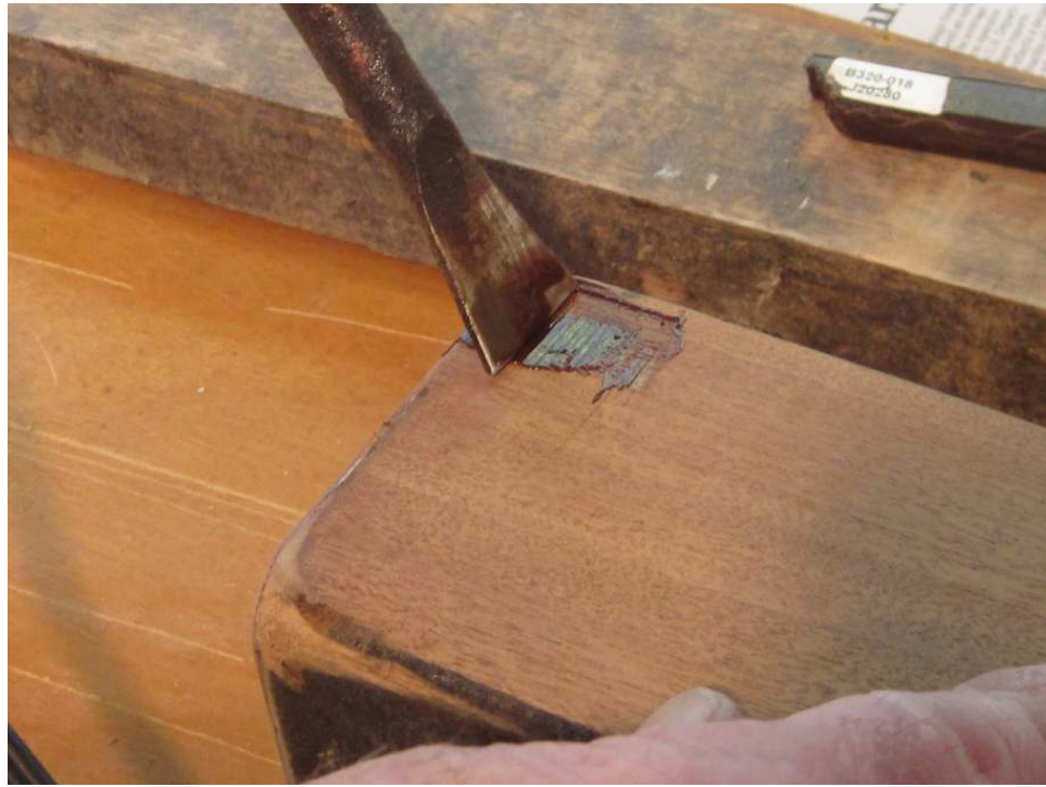
Photo 26: Lacquer stick is used here to fill in a gouge in the veneer. A darker shade than the raw wood is necessary, since the lacquer stick is not affected by stain. The repair should match the finished color of the wood, not the color of the unfinished wood.
