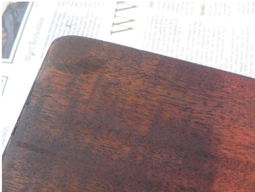
Photo 29: The repaired area now blends in with the rest of the veneer. After the top coats of polyurethane are applied, it will be less noticeable yet.
