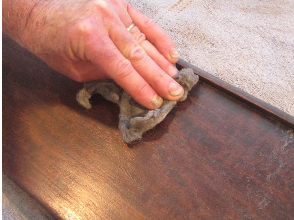
Photo 31: After being sanded, the final coat is then buffed out with 0000 steel wool. Basically, the glare is scrubbed off, leaving an even satin finish, ready for polishing.
