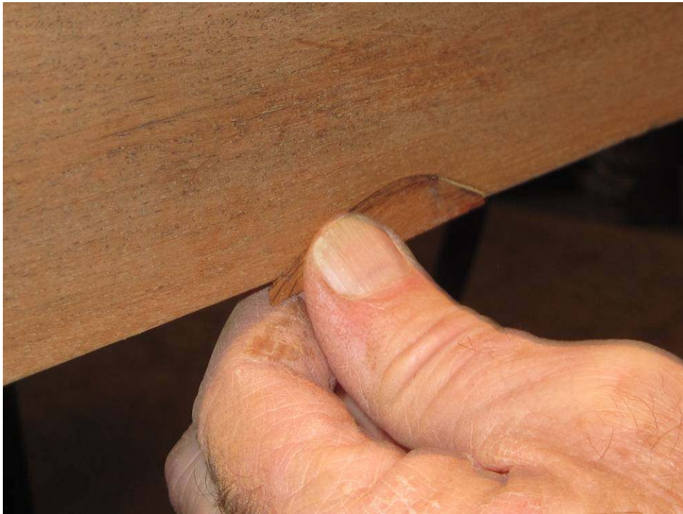
Photo 25: Damage to case needs repair. Here Dave works on fitting a veneer patch for a damaged area. The underlayment and veneer will be glued in place with hot animal hide glue, then sanded out. If done right, this repair is virtually invisible once finished.
