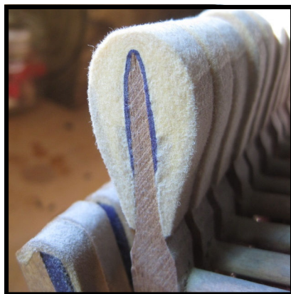
Worn hammer after filing
