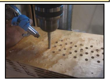
Once the panels have been drilled for size #2 pins, they are installed in the routered out sections and glued in place. At that time the cast iron plate is positioned back in place and bolted down (photo below).
