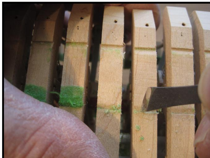
When the old felts have been removed and the undersides of the wippens cleaned, new high-quality abstract felt is carefully glued into place. These felts are glued at the front and the back, but not in the center, so that the transmission of sound between the brass capstans and the wooden parts of the action is kept to a minimum.
