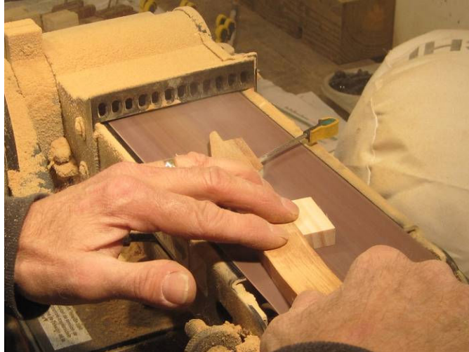
Photo 7: Sanding the sides flush.
