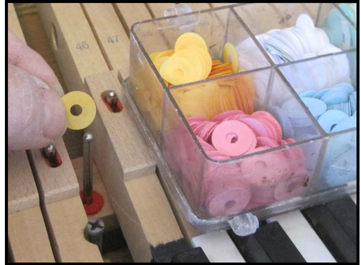
.002" paper punching being installed
