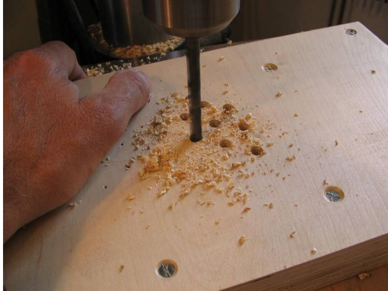
Photo 6: Drilling through the press.
