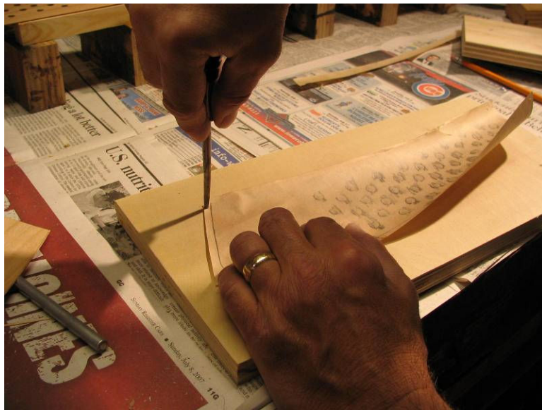
Photo 3: Marking the positioning holes on the press.
