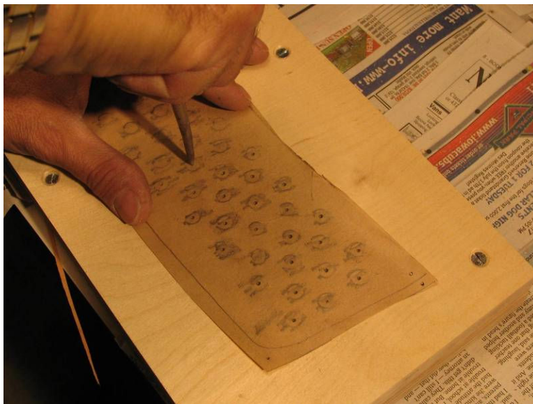
Photo 5: Marking the location of the tuning pin holes.
