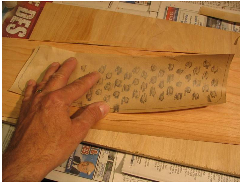
Photo 2: Transfer of pattern markings to veneer.
