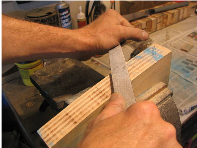
Photo 4: Filing off the high spots.
