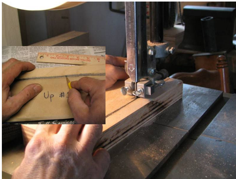
Photo 1: Cutting the panel on the band saw.
