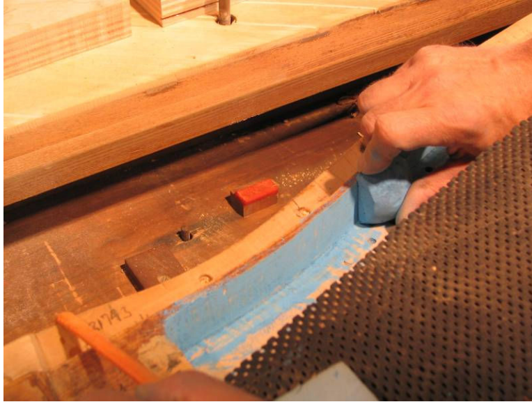
Photo 2: Chalking the wall of the cavity.
