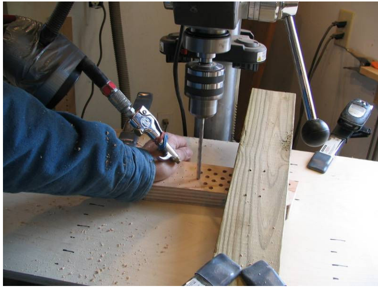
Photo 8: Drilling the panels.
