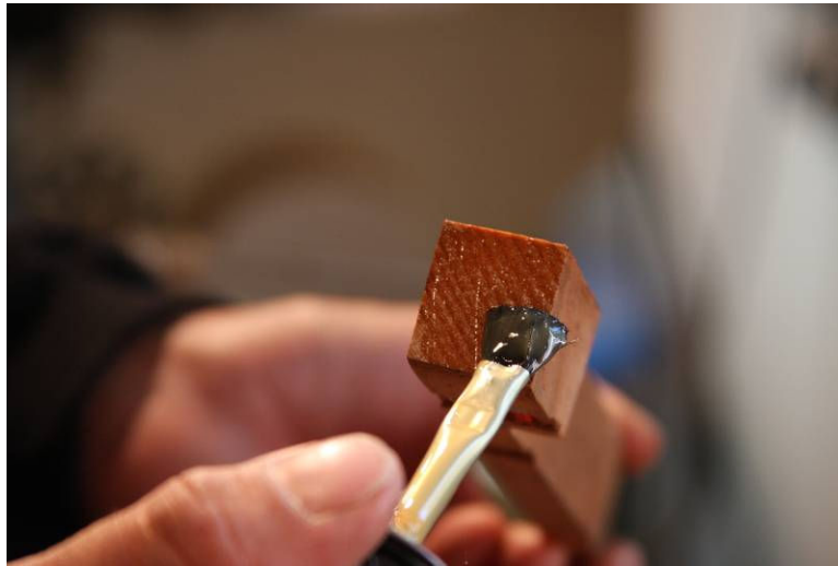
Photo 2: Apply glue to the front of the keystick.
