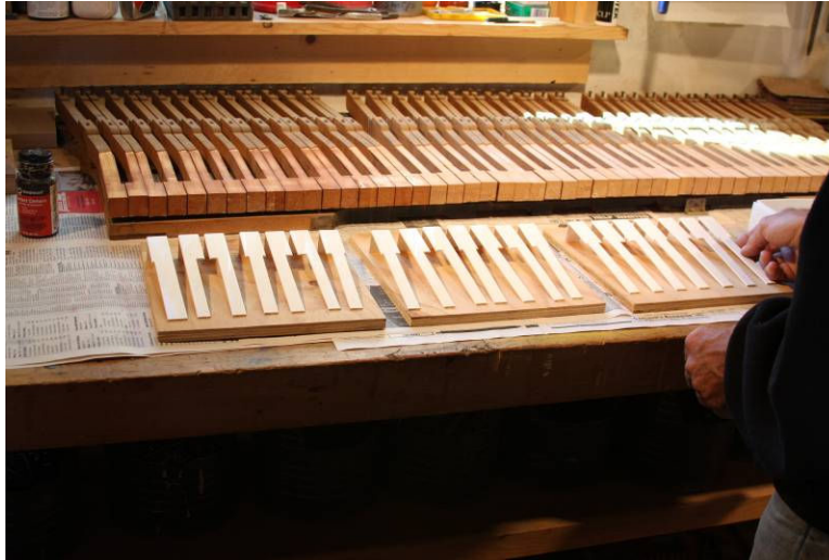
Photo 3: Plywood squares hold an octave of keytops.
