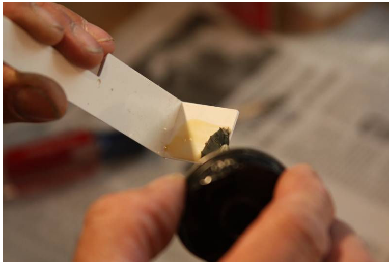
Photo 4: Begin gluing with the inside of the keyfront.
