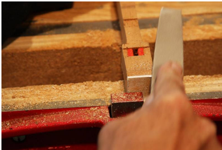
Photo 10: Filing off the excess.
