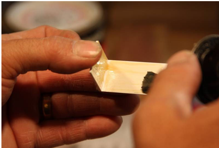
Photo 6: Applying glue to the underside of the keytop.
