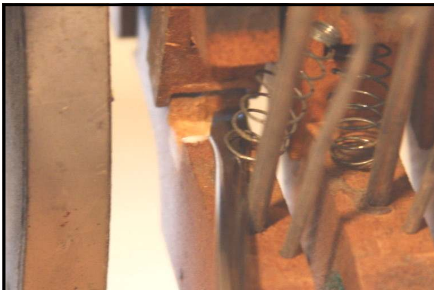
Photo 4: Application of glue to mortise.
