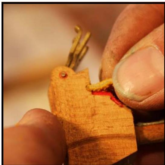
**Step 31:** Once the hot glue is applied, quickly insert the end of the hammer butt buckskin into the slot. Make sure that the fit is tight on both the left and right side. Let glue cure for 10 minutes or more before going to the next step.
