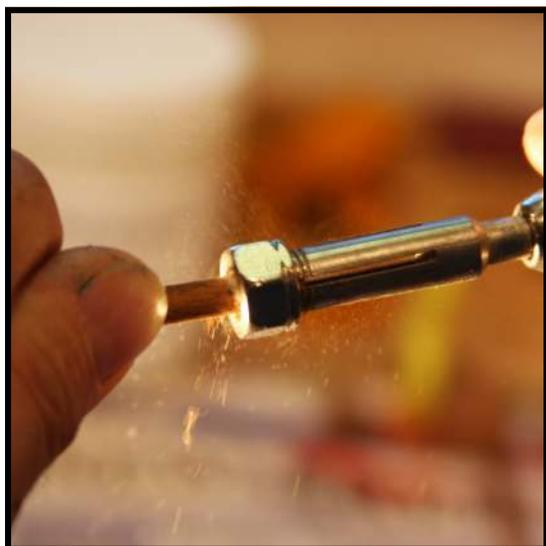
**Step 1:** As you remove hammer butts from the action, number them in order, starting with #1 for A0 to #88 for C8. Then, remove the remains of the hot glue from the hammer shanks (if the old hammers have been removed) using a [hammer shank reducer \(Cat. No. 75\)](#) along with a [combination tool handle \(Cat. No. 26\)](#). Turn the nut on the reducer to remove just the glue, and none of the wood of the hammer shank.
