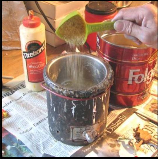
**Step 13:** With all the felt and leather removed from the hammer butt (the center pin bushings were not replaced on this particular piano), it's now a good time to prepare for installation of new materials used in restoring the hammer butt. First, a small batch of hot animal hide glue should be prepared, using an [electric glue pot \(Cat. No. G-1155\)](#), and [dry cabinet glue \(Cat. No. 399-1/2\)](#). Use slightly more water than glue for the correct consistency.
