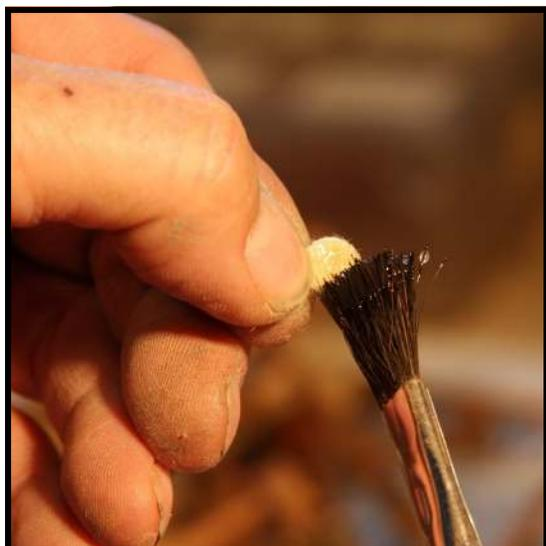
**Step 22:** Stir your hot glue again with the hammer shank. It should be the consistency of honey with the pot set at 160 degrees. Use a [glue brush \(Cat. No. 438\)](#) to apply a small amount of hot glue to a [spring punching \(Cat. No. 330E\)](#). If you're unable to grip the felt by the edge with your fingers, use the pointed end of a pair of [needle nose pliers \(Cat. No. 239\)](#) to grasp the felt while the glue is applied.
