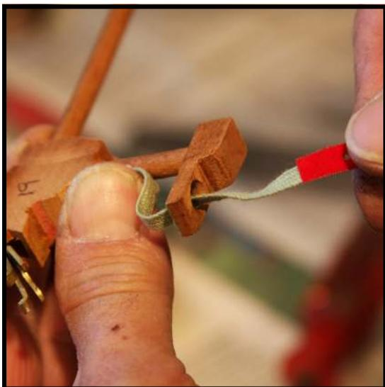
**Step 20:** Holding the end of the bridge pin firmly in place for a moment, pull the excess of the bridge pin on through the hole in the catcher.
