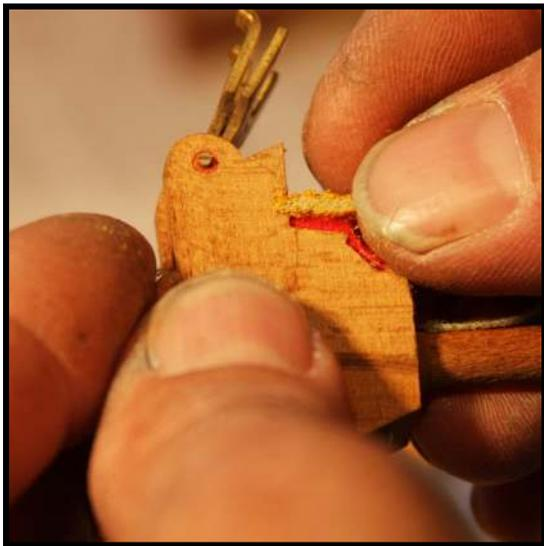
**Step 29:** When you've achieved a snug fit, you're ready to glue. The buckskin is glued into the slot on the one end, and to the wood of the hammer butt on the other end. It is not, however, glued to the underfelt in between those two points, but rather stretched over the felts at tension.
