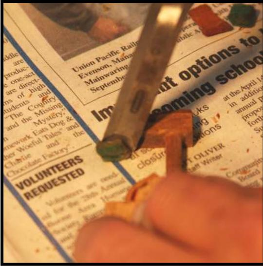
**Step 4:** With the flat edge of your 1/2” chisel up against the underside of the catcher, shave off the catcher felt. A pivoting motion, with the corner of the chisel against the bench, works best. The chisel must be sharp for this operation and even so, there may be felt and glue residue which remains. Be cautious not to remove wood from the catcher in the process. You will clean up any residue with a file in a later step.
