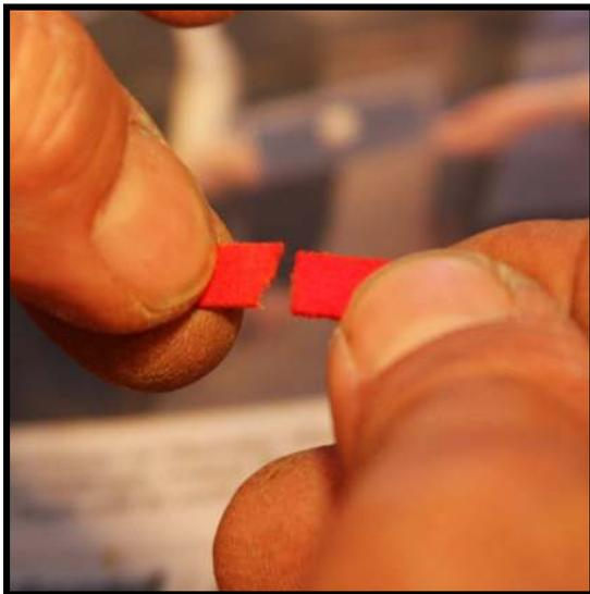
**Step 17:** Before cutting any more pieces of felt, visually compare the new piece of underfelt to the old. If the two don't match exactly, make an appropriate adjustment on the felt cutter.
