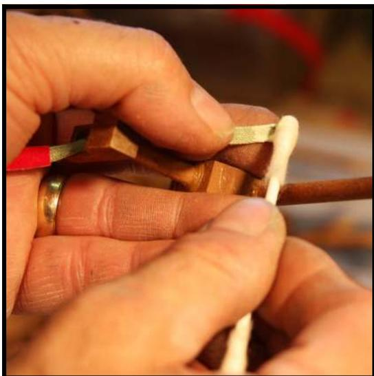
**Step 19:** Insert the bridge pin through the hole in the catcher. Holding the hammer butt as shown, with your middle finger supporting the end of the bridge pin, apply a drop of [Titebond glue \(Cat. No 392-4\)](#). A small amount put in a bottle cap, then applied with a Q-Tip, makes for less mess than using out of the squeeze bottle.
