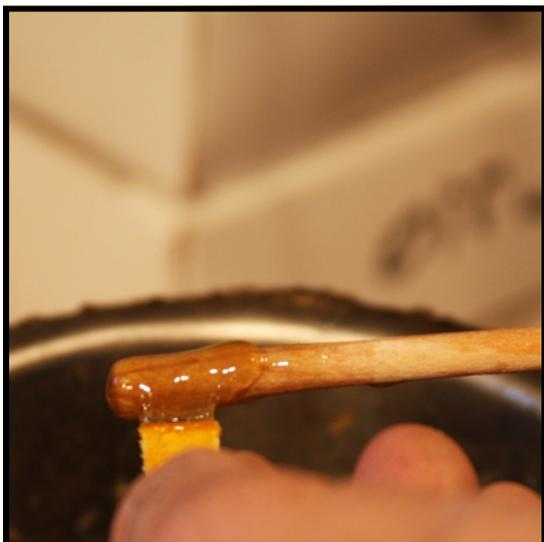
**Step 30:** Apply a small amount of hot glue to the correct end of the hammer butt buckskin using a hammer shank as an applicator. Make sure you have glue on both sides and on the very end of the piece of leather.
