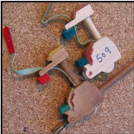
**The Options:** To properly restore this piano, either outright replacement of the set of hammer butts, or complete restoration of the original butts with a replacement of all leather and felt was necessary. The choice came down to balancing the cost of replacement against the time required for stripping and replacing the old felts and leathers.
