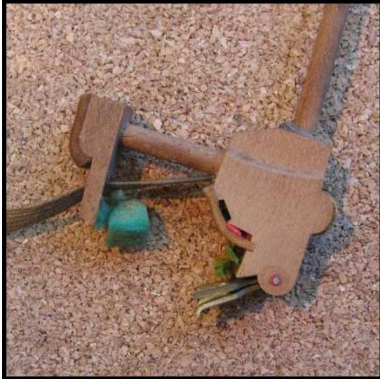
**The Problem:** Insect damage and wear would make fine regulating of the subject piano very difficult. Hammer butt felts were missing or damaged. The catcher buckskins were worn very thin, in places down to the wood. The most problematic situation was with the felts under the hammer butt buckskin. In places the underfelt was missing either partially or altogether. Plumping out with yarn would not be effective because of this inconsistency.
