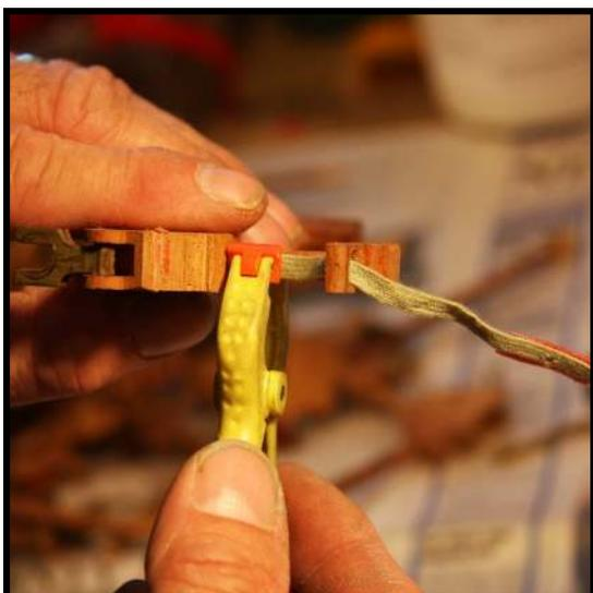
**Step 21:** Use a small clamp to hold the bridge pin in place for 5 minutes or more.
