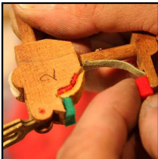
**Step 38:** Apply hot glue to one half of a side of a hammer butt felt, and press into place below the bridle strap hole in the catcher.
