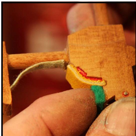
**Step 37:** Apply hot glue to a square cut from a strip of [hammer butt felt](#) (Cat. No. 307, 308 or 309), and press firmly into place below the hammer butt buckskin.
