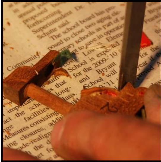
**Step 7:** Turning the hammer over to the opposite side, use your chisel to slice off the hammer butt felt with one clean stroke.
