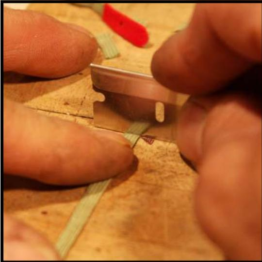
**Step 14:** If any of the original bridle straps are intact, measure the length of one from where it emerges from the catcher shank, and cut your new [original standard bridle straps \(Cat. No. 1515\)](#) to the same length. [Cork bridle straps \(Cat No. 6516S, M, or L\)](#) are an option. (While completing these other steps, go back to your glue pot occasionally and stir your glue with a hammer shank.)
