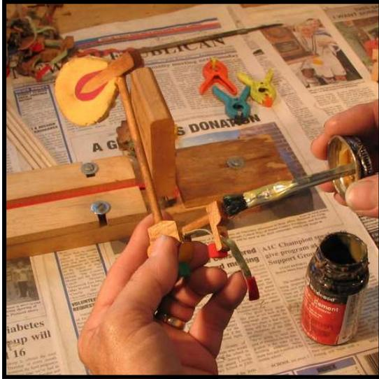
**Step 34:** Cut catcher buckskin approximately to size. Apply contact cement to both the catcher and the buckskin and allow to sit for at least 15 minutes, or until tacky. An alternate method is to clamp together a number of hammer butts with the catchers in line and to glue a strip of buckskin over the catchers from one end to the other.
