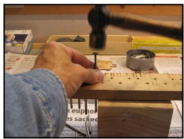
In the photo to the left, balance rail pins are shown being tapped out from the underside of the balance rail. Again, care is taken not to damage the original hole. The old pins will be measured with a micrometer to determine their exact size. The new pins, when they are driven in, will be tight as long as care has been taken in removing the old pins. What are the basic procedures for installing a replacement set of keypins?
