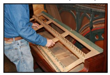
The keys need to be removed from the piano to access the keypins. Additionally, the keyframe itself is typically removed so that the repair work may be done on a workbench. In the case of a grand piano, the action is removed, then the upper stack is taken off of the action to access the keys.
