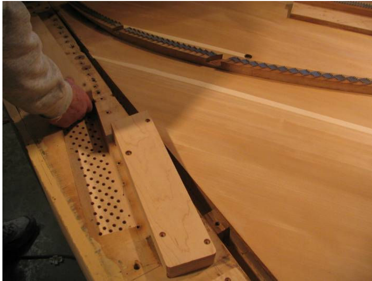
Photo 5: Fitting the panels
