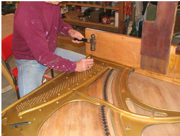
Photo 6: Using a centering punch to mark the panels for drilling
