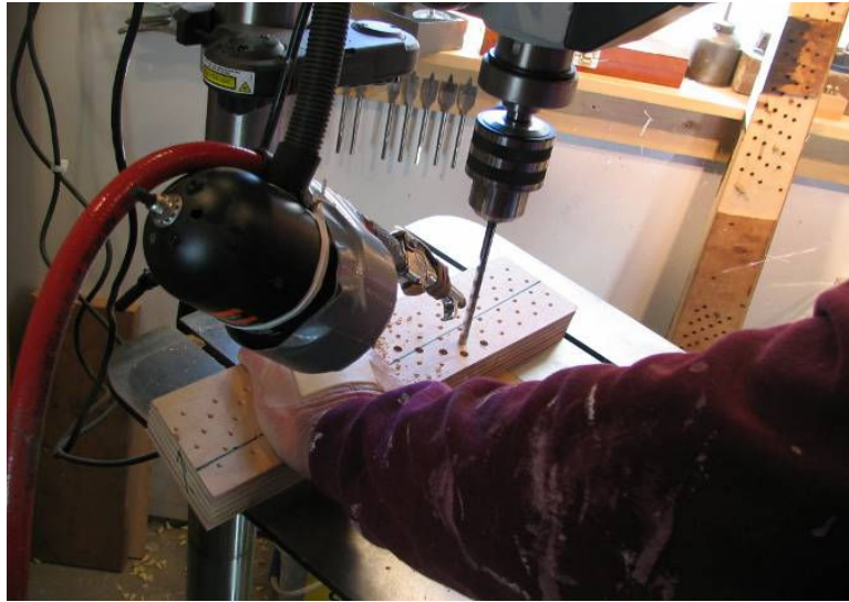
Photo 7: Drilling the pinholes in the panels
