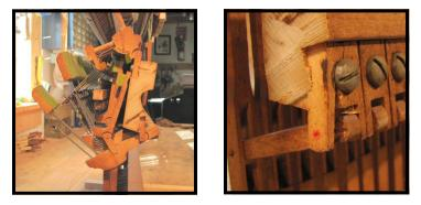
**Further explanation of need for repair:** If the action of an upright piano is removed for servicing and a bridle strap is broken or missing, the lower portion of the mechanism (the wippen) will swing down (left photo).
