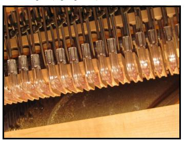
If you would like to have a new set of Vagias Snap-On Elbows installed, contact me at your convenience to set up an appointment. Working together, we can make sure that your piano is maintained correctly for your maximum enjoyment.
