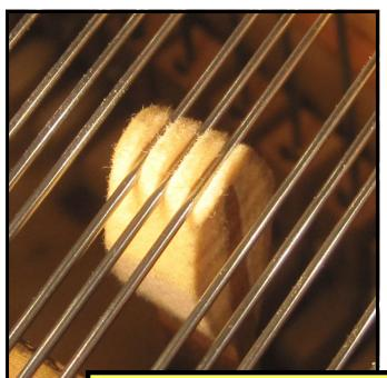
When a hammer with deep cuts from years of hard playing strikes the strings it has a mushy feel. The felt of the hammer, instead of delivering a clean blow to the strings, wraps around the strings upon point of impact producing an unsatisfactory tone.
