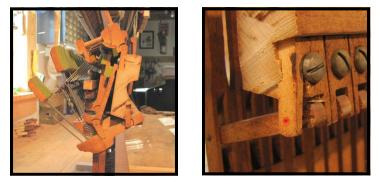
**Further explanation of need for repair:** If the action of an upright piano is removed for servicing and a bridle strap is broken or missing, the lower portion of the mechanism (the wippen) will swing down (left photo).
